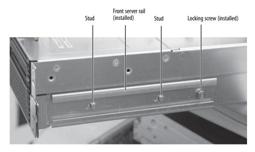
2 Align the locking screw holes in the rails with the threaded screw holes in the server, then install one locking screw through the each front server rail. 3 Align the slots in the back server rails with the studs on the side of the server, then engage the slots with the studs and slide the rail forward until it stops.
